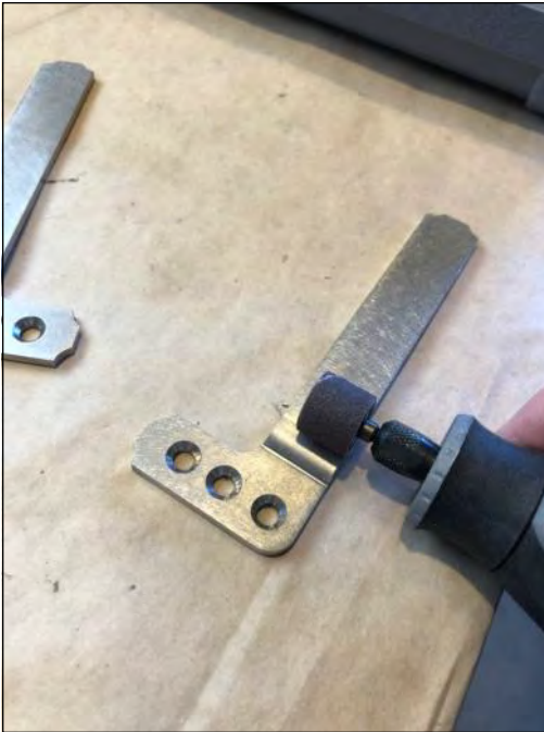
Using the Dremel tool to sand out the tooling marks
