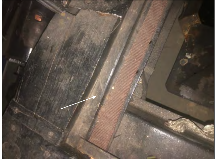
Left: extra threaded D-Nut location for floorboard screw on the Tudor Sedan. Right: Recessed area in wooden side sill on Cabriolet to support the front floorboard, with no screw location for floorboard.
