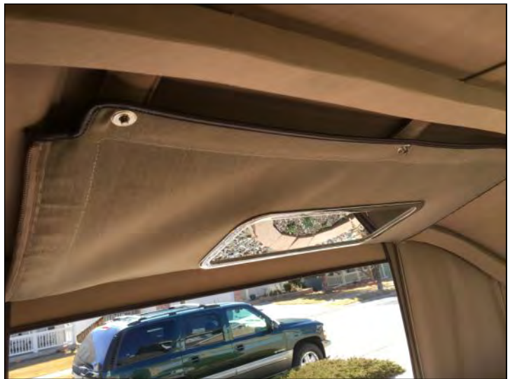
Rear top panel and Curtain Light in the "Ventilation" position.
