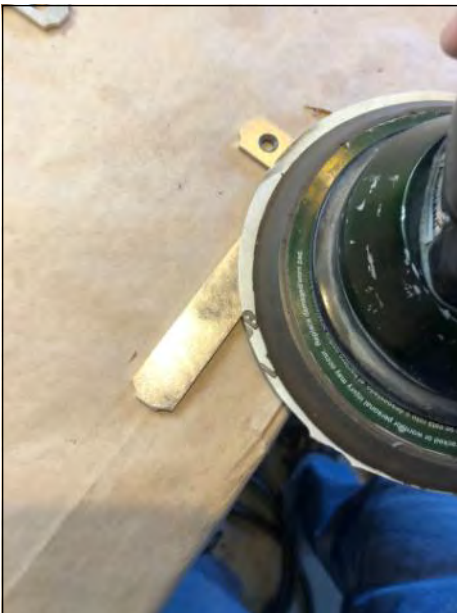
Smoothing out the Dremel marks with 220 Grit sandpaper and an orbital sander.
