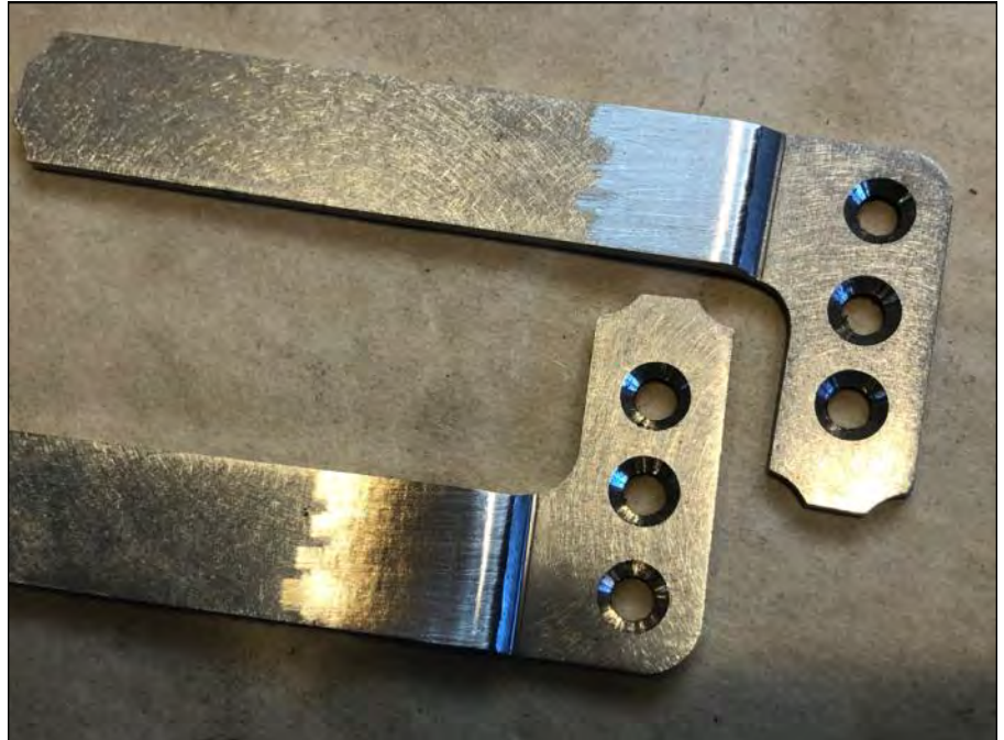
Tooling marks are removed. Be careful not to round off any edges or corners.
