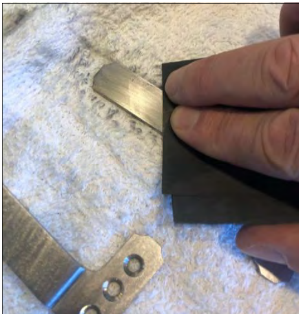
Sand in one direction on the part. Keep the sandpaper “wet” with Alumicut.
