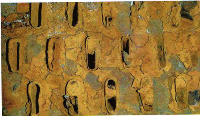
Fig. 4. Radiator that was tanked only. Tanking did nothing to clean this radiator.
