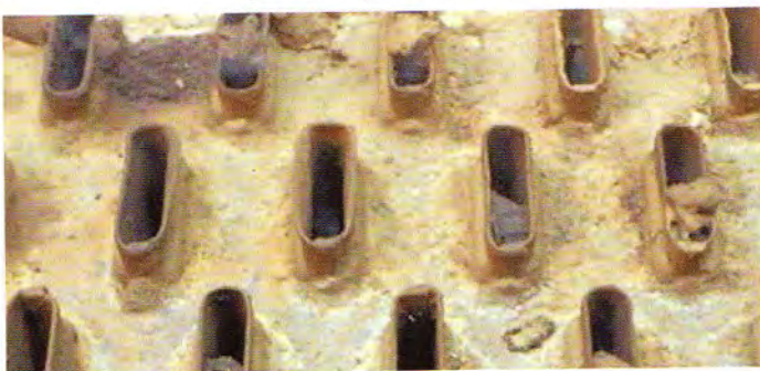
Fig. 5. My radiator that was tanked only. Radiator was still about 1/3 restricted.
